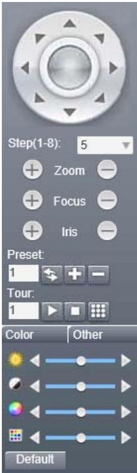
In this window you manually control the camera movements, automatic movement and image settings.
